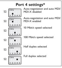
\* Setting of port 4 is only possible when using SDW-541.
